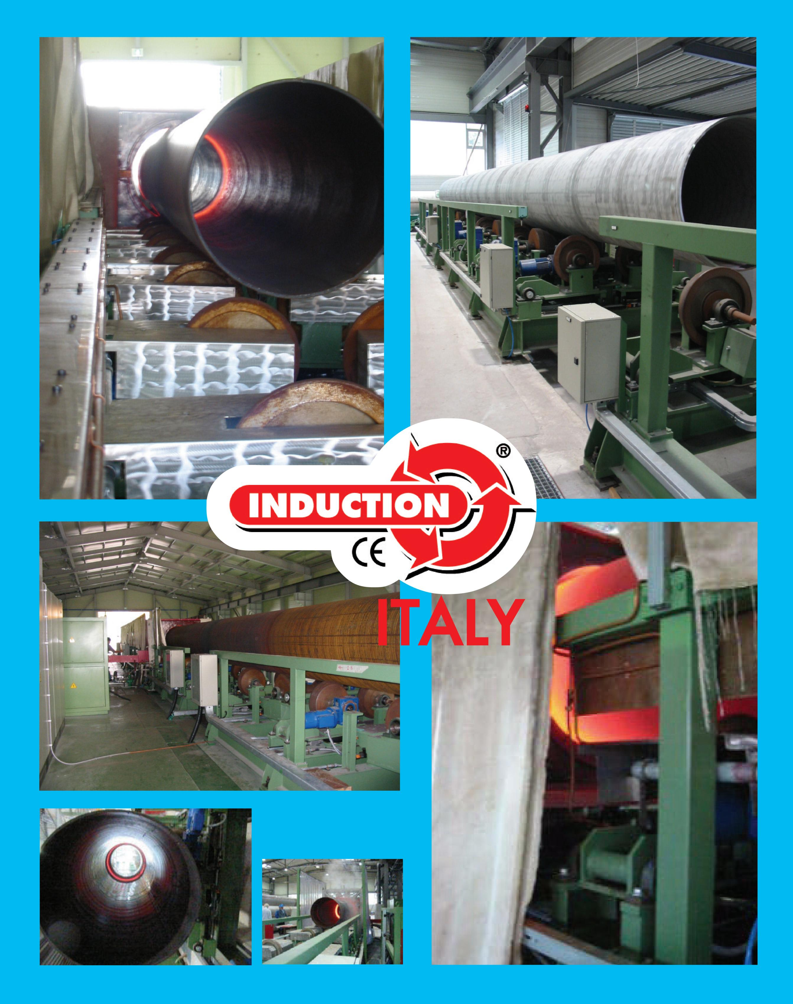
2 MW SOLUTION ANNELING AND HEAT TREATMENT LINE FOR STAINLESS STEEL AND CARBON STEEL PIPES
