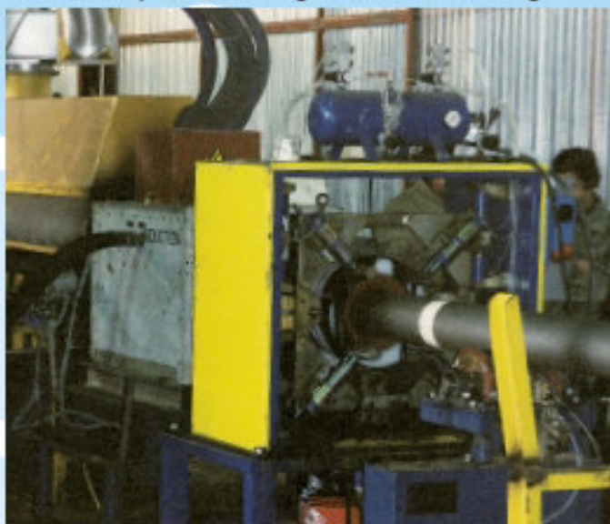
Impianto da 1000 KW per rivestimento a calza 1000 KW plant for ring extrusion coating
